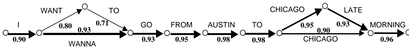
Figure 2: Word-graph generated for the example in Figure 1. The bold arrows indicate the best hypothesis.
